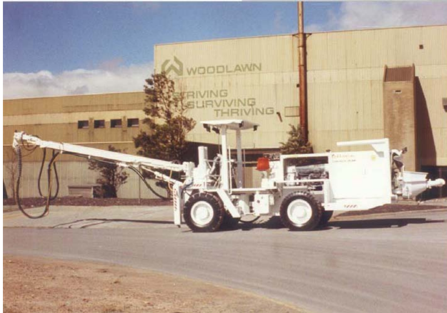
Figure 10 - Purpose Built Woodlawn Shotcreter 1995
