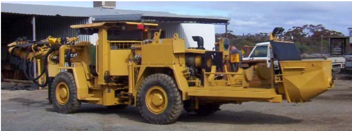
FIG 7 - Lightning Nickel Shotcreter. Atlas Copco 282 carrier
