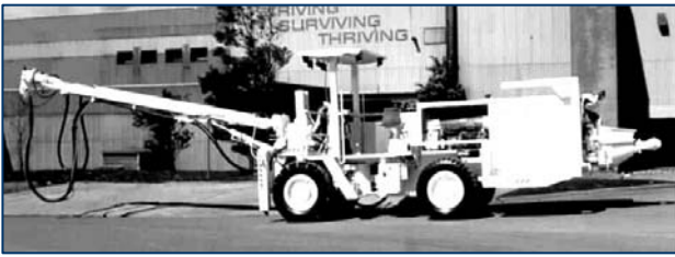
Plate 1. Modified Jumbo based Shotcrete Machine
